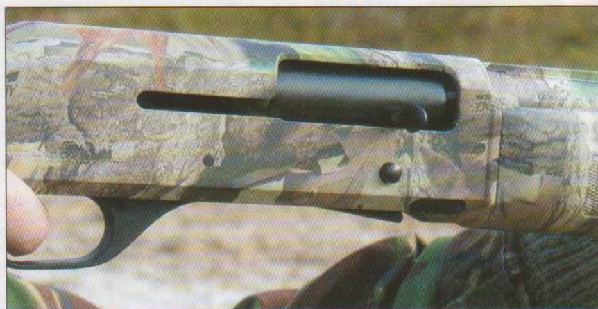
Receiver detail showing the bolt release catch and bolt in battery, the camo finish is well applied and matches nicely
